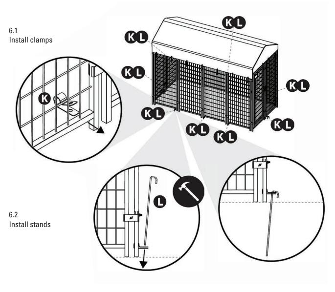
Note: If kennel is on a hard surface such as a deck or patio, use lag or concrete screws with clamp.
